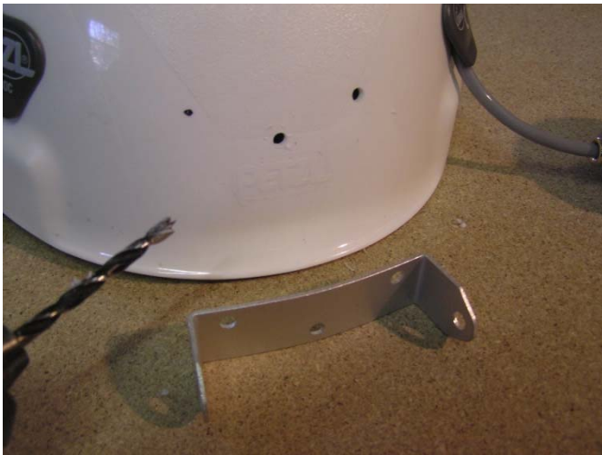
Prepared drillings for the lamp holder
