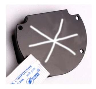
Fix the heat sink using four screws and remove excess thermal grease.
