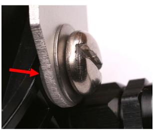
When reinserting the screws, do not over tighten them! Doing so will damage the spring washers (red arrow). Make sure the conical spring washers are mounted correctly, see orientation in image!
